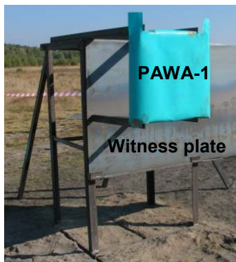
Fig. 7. PAWA-1 armour on the stand with steel witness plate
