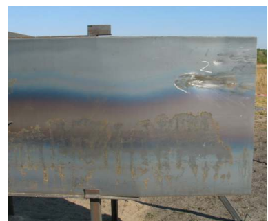
Fig. 9. Steel witness plate after 2nd firing
