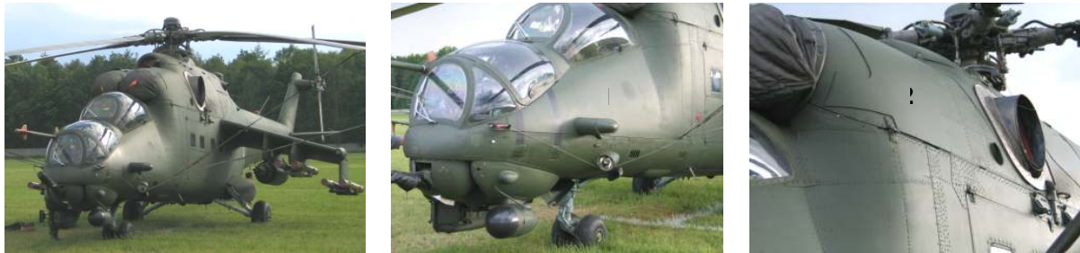
Fig. 2. Polish gunship - Mi-24W helicopter with the additional protection of the cockpit (1) and the engine (2) against the perforation with 7,62 mm armour-piercing projectiles
