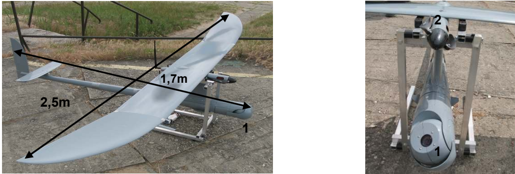
Fig. 9. View of SOFAR UAV with camera (1) and electric propulsion (2)
