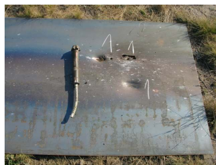
Fig. 8. Steel witness plate after 1st firing
