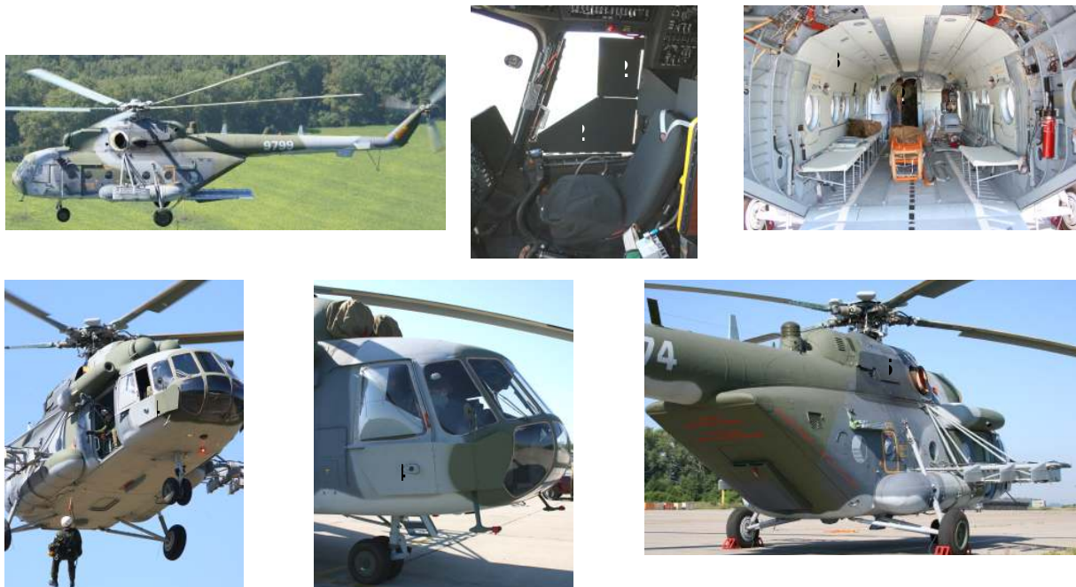
Fig. 3. The Czech gunship Mi-171Š with the additional protection of the pilot seats (1), windows (2), the cabin (3), the cockpit (4) and the engine (5) against the perforation with 7,62÷12,7 mm armour-piercing projectiles
