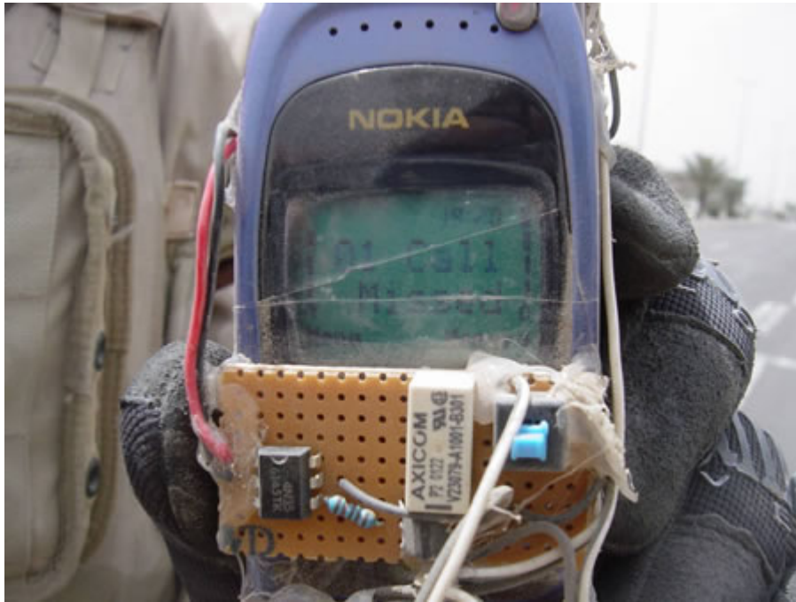
Picture of cell phone used to trigger an IED. Source: LiveJournal.com
